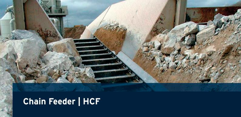
■ Chain conveyors are successfully used in different branches and applications. Especially coarse or cohesive material as usually occuring in mining and mineral processing, is continuously and smoothly transported with a chain conveyor. Being used as a discharge conveyor under bins and bunkers the chain feeders take up large static and dynamic loads, if for example fed with large feed sizes or from a greater height.
