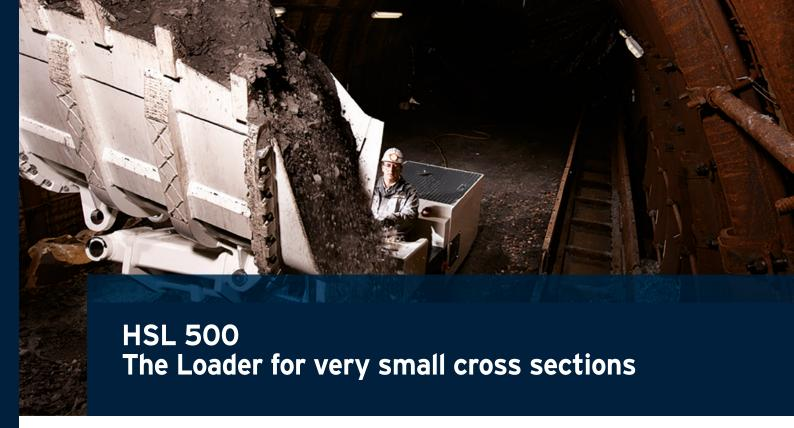
The HAZEMAG side tipping loader HSL 500 with a bucket capacity of 0.6 m³ is the reasonable loading machine for small and very small cross-section roadways.
