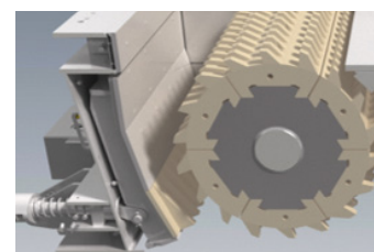
Adjustable and retractable crushing wall
