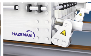
Adjustable and retractable crushing wall
